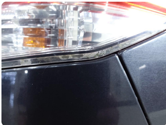
4.2 Krakelering i plast
