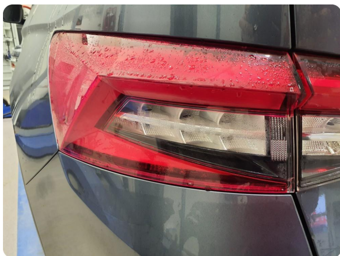
4.2 Dugg/fukt Fukt I baklampe
